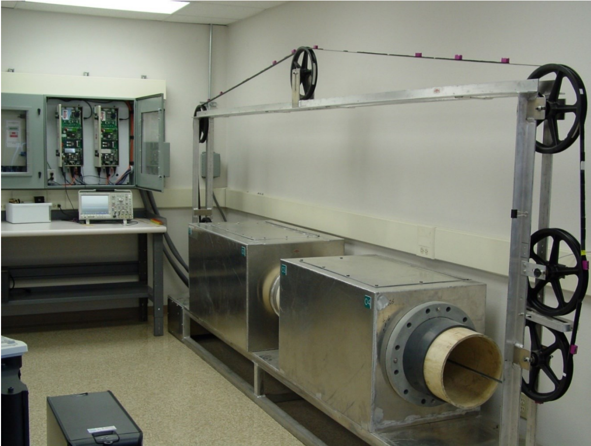
Figure 3. Configuration of belt, antennas, and tag groups for separation test.
