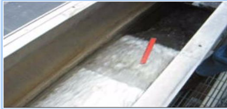
Figure 6. A slide gate diverting a test PIT tag.
