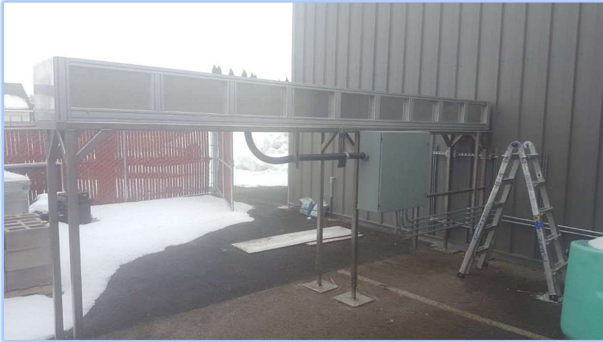
Figure 15. Motorized, PLC-controlled tag transport located outside of the room
