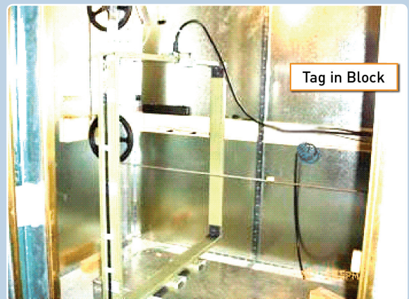
Read-range distances were measured with tags placed along the Z-axis out from the center of an antenna.
