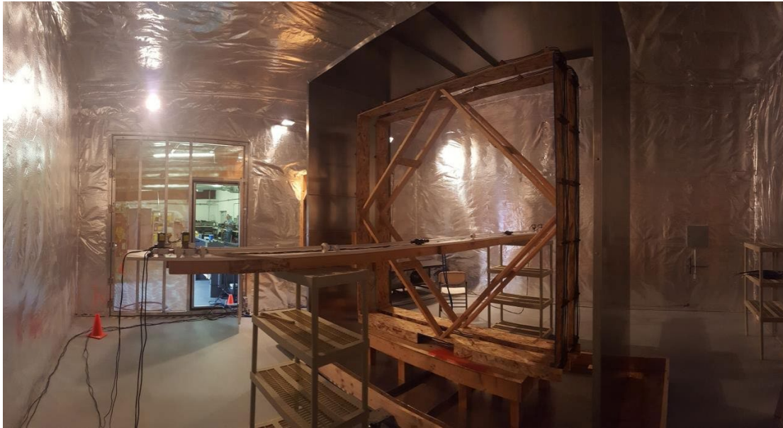
Figure 2. Photo of the \frac{1}{2} -scale model of the BCC antenna. Note the RF shielded room, aluminum shield and pneumatic shuttle for passing the PIT tag through the antenna automatically.
