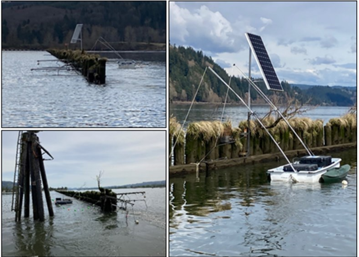
Figure 3. Pile dike PIT interrogation sites equipped with solar panels, electronics barges, antenna brackets, and antennas. Clockwise from top left: site PD6, barge at PD8, antenna orientation at PD5.
