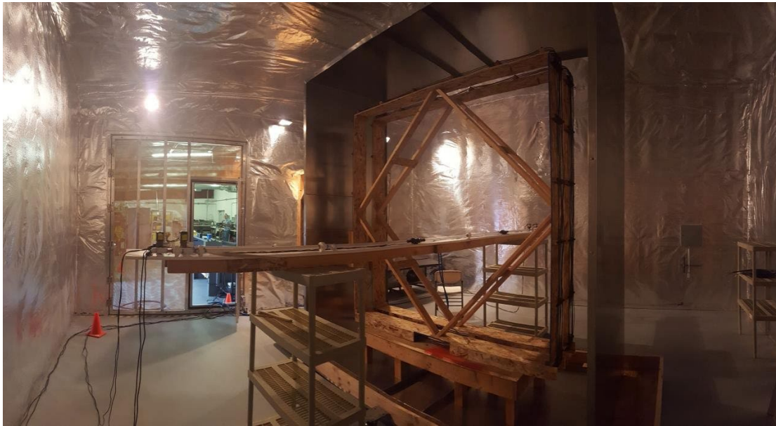
Figure 2. Photo of the 1/2-scale model of the BCC antenna. Note the RF shielded room, aluminum shield and pneumatic shuttle for passing the PIT tag through the antenna automatically.
