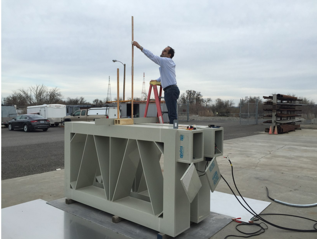
Smirnov measuring read range of initial ogee antenna.
