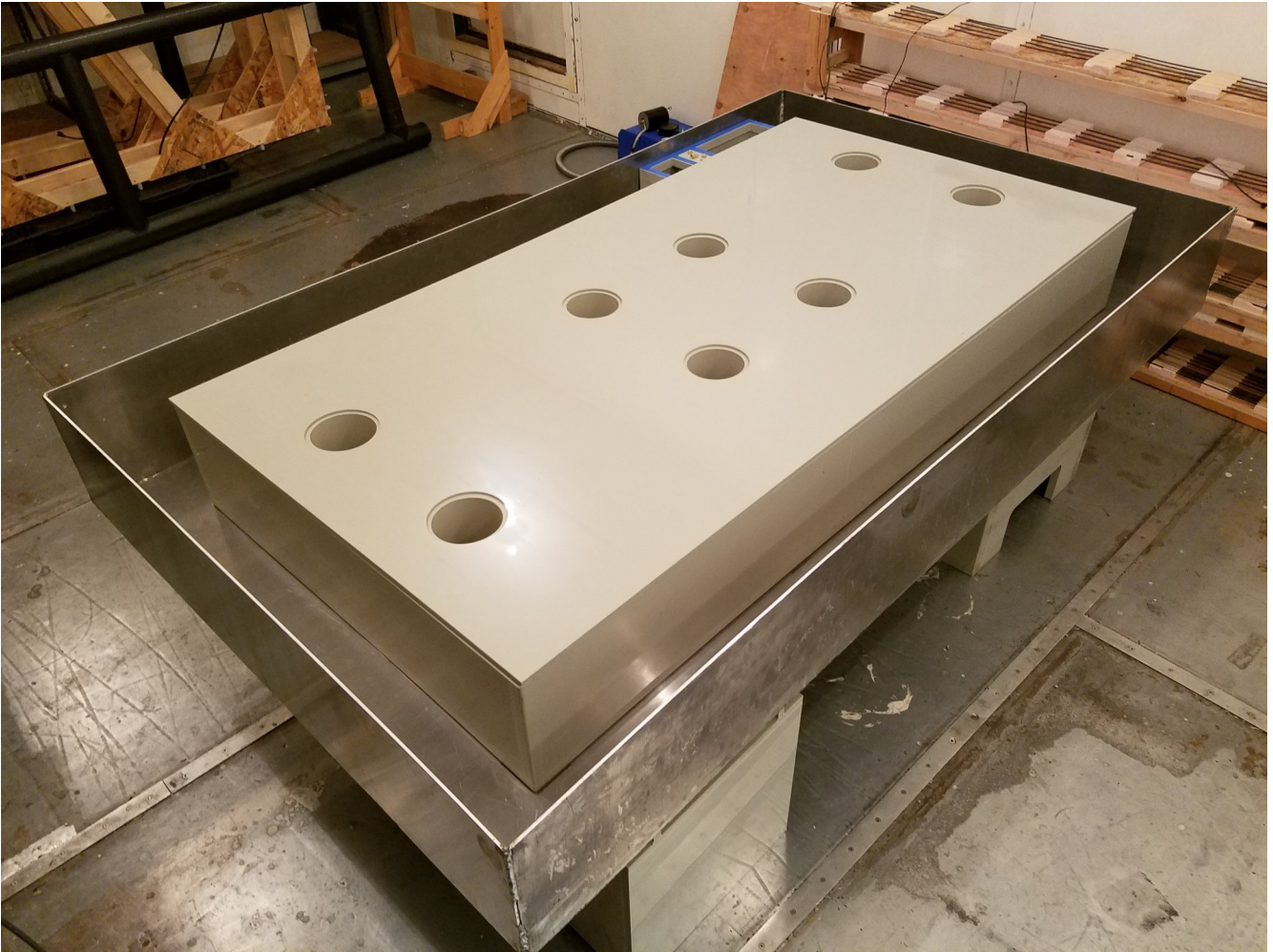
Figure 4. Completed ogee antenna and external aluminum shield.
