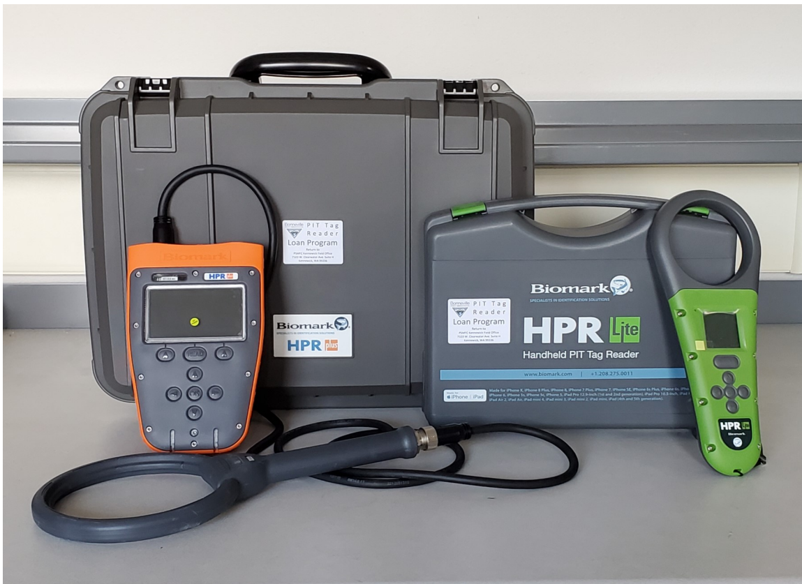
Figure 1. HPR Plus and HPR Lite PIT tag readers.
