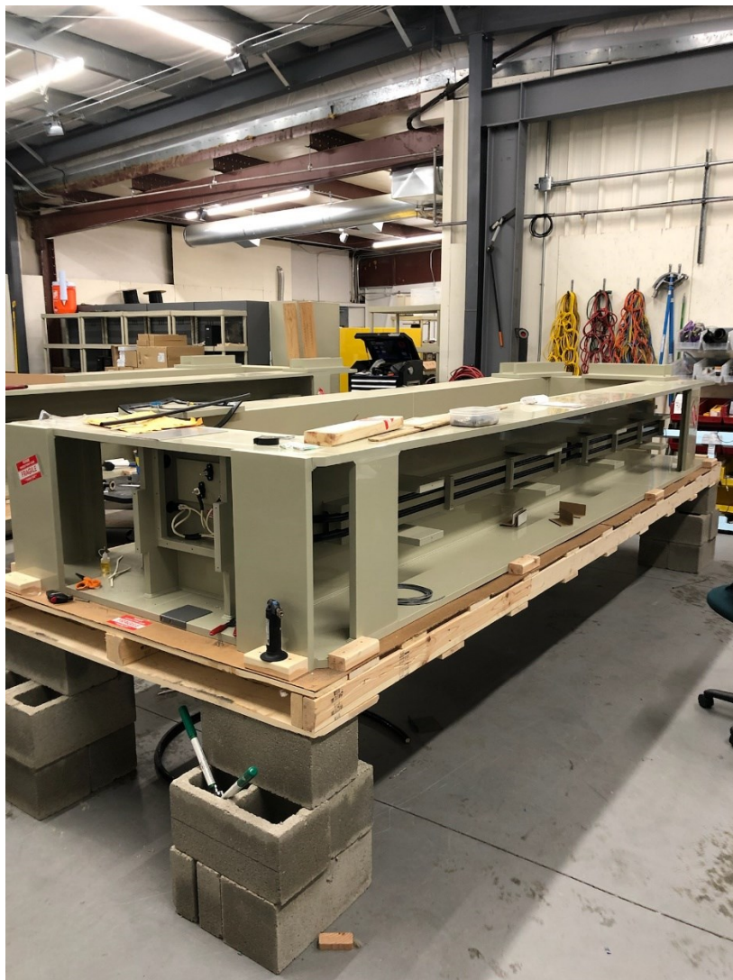
Figure 9. BO4 PIT tag antennas under construction at the Kennewick lab.
