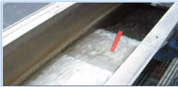
Figure 7. A slide gate diverting a test PIT tag.
